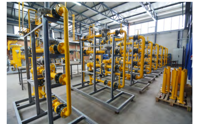
B. Palanka for the company Novi-Sad Gas Ltd. (Serbia) REGULATING STATIONS Q = 2.500 \text{ m}^3/\text{h} | p = 12 \text{ bar}
