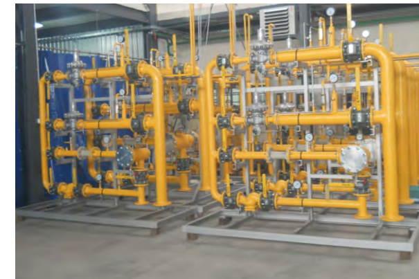
B. Palanka for the company Novi-Sad Gas Ltd. (Serbia) REGULATING STATIONS Q = 2.500 \text{ m}^3/\text{h} | p = 12 \text{ bar}
