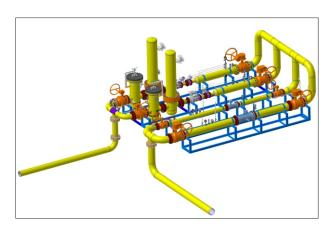
MAIN REGULATION - MEASURING STATION Q =  $40.000 \text{ m}^3/\text{h} \mid \text{p} = 50 \text{ bar}$  Control cabinet - FLOW COMPUTER for MAIN REGULATORY - MEASURING STATION
