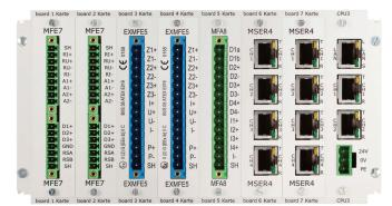
ensured that the required Ex-barriers are fitted in the control cabinet. They are not needed when using Ex-d sensors instead. In addition, the MFE7 can ensure the voltage supply to both current inputs and thus reduce the amount of wiring required. The HF inputs can be configured to work with pulse integrity checking according to ISO 6551 Level A.
