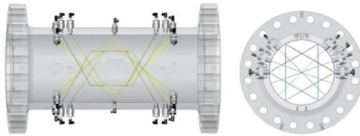
The TwinSonic<sup>plus</sup> is a combination of the Q.Sonic<sup>plus</sup> and the CheckSonic 2-path in one meter body. The Q.Sonic<sup>plus</sup> uses two pairs of double and two single reflection paths. Taking the mean value of both pairs will result in a symmetrically weighted measurement. The subtraction of the paired paths provides an indication of asymmetric flow along the mirror plane of the paths as an additional diagnostic feature.
