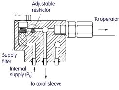
As the operator opens, a flow and hence pressure drop is created across the restrictor. The pressure drop is transferred directly to the back of the axial sleeve.
